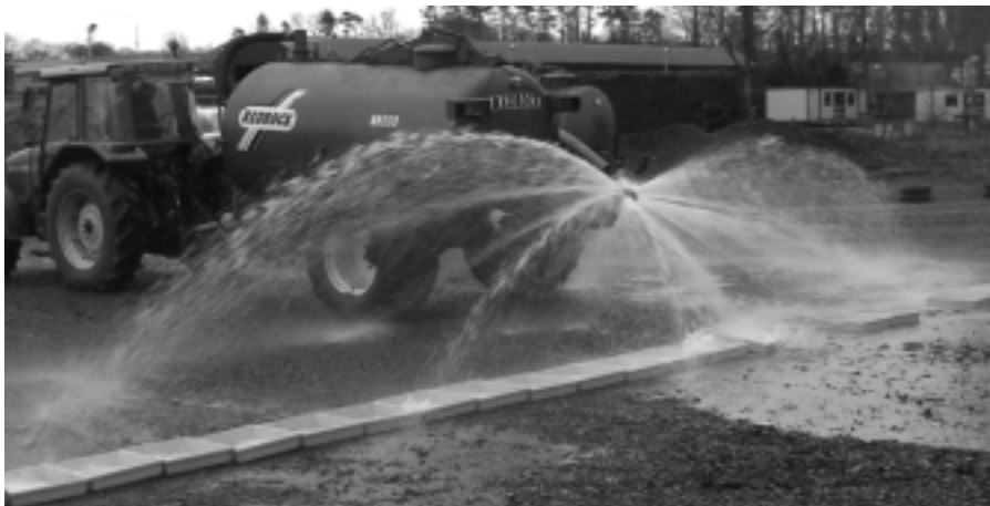
Figure 4: Uneven application is visually evident from this used splash plate
